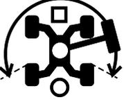
Light on indicates that the boom has moved past a circle-end tire and the drive function has been interrupted. To drive, move the drive enable switch and slowly move the drive control handle off center. Use the color-coded direction arrows on the platform box and drive chassis to identify the direction the machine will travel.
