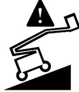
**Machine Not Level Light Flashing:** If the tilt alarm sounds when the platform is raised, the Not Level indicator light will come on and the drive function in one or both directions will not operate.
